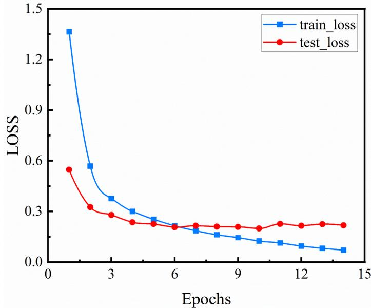
Fig. 5 Changes in loss during the training process of the XLNET model over time
