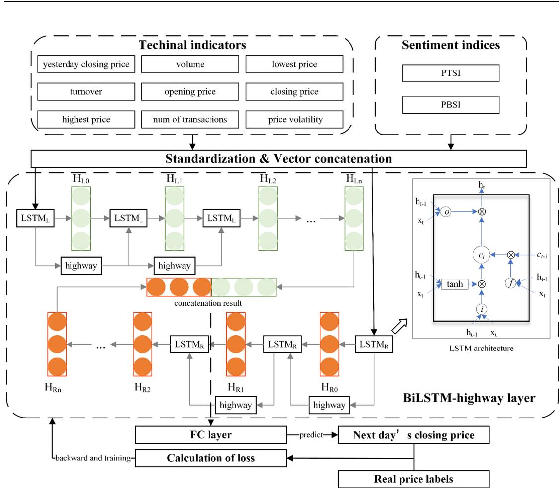
Fig. 3 The BiLSTM-highway module structure for stock closing price prediction
