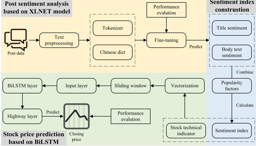
Fig. 1 The structure of XSI-BiLSTM.
